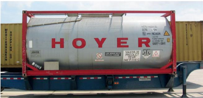
Tank containers or demountable tanks are used for safe road, rail or water transport of aggressive or ultra-pure media. Quality requirements with regard to the component are very high as hazardous materials are transported via public traffic routes. For this purpose, Plasticon Composites supplies special trailers in composite design (FRP with thermoplastic and fluoroplastic).
